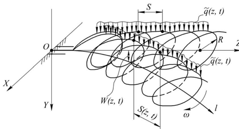
**Fig. 2. Equivalent scheme of the spiral spring oscillation potato heap separator**
