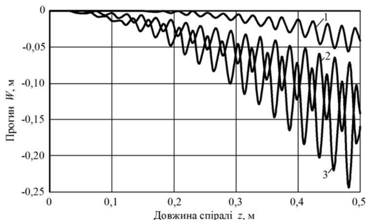
**Fig. 3. Dependence of complete deflection  $W$  the spiral axis from its length  $z$  with its own bending oscillations and the action of evenly distributed load: in moments of time: 1 –  $t = 0$  s; 2 –  $t = 0,05$  s; 3 –  $t = 0,25$  s**
