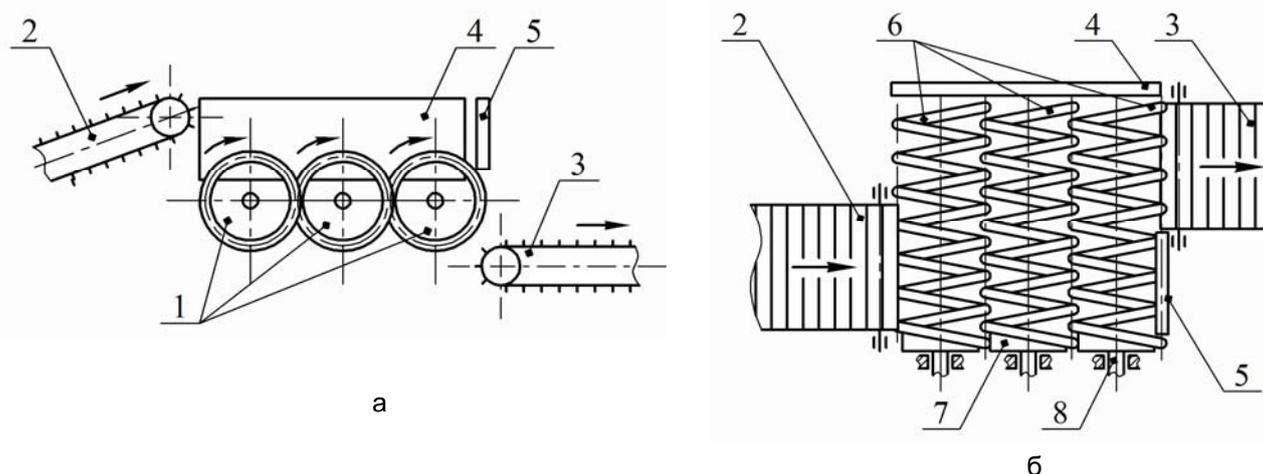
**Fig. 1. Spiral potato heap peeler dug out of the soil:**
