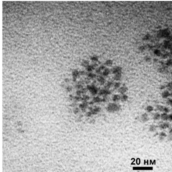
**Fig. 3. An electronic micrograph of quantum dots of cadmium selenide**
