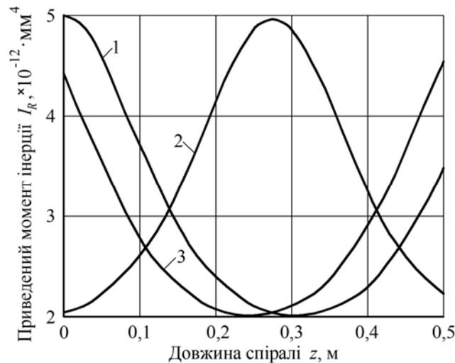
**Fig. 3.** Change on the length of the helical moment of inertia  $I_R$  section of a console with a spring diameter  $d = 17$  mm, winding pitch  $S = 48$  mm, upward winding angle  $\gamma = 7^\circ$  and the angular velocity of rotation  $\omega = 30$  rad. $\cdot$ s $^{-1}$  in moments of time: 1 –  $t = 0$  s; 2 –  $t = 1$  s; 3 –  $t = 2$  s
