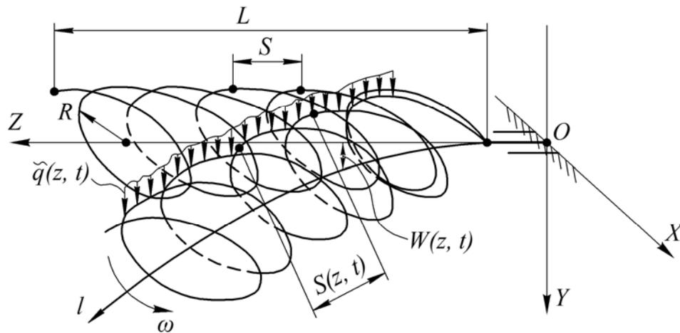
**Fig. 2. Equivalent scheme of spiral spring oscillation under the influence of external variable load from the side of the potato heap**
