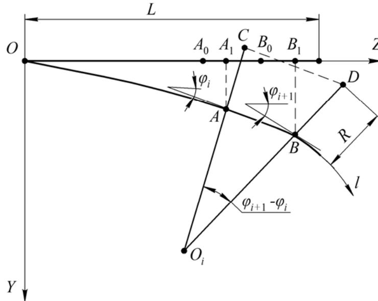
**Fig. 4. Calculation scheme of cantilever elastic spiral bending**
