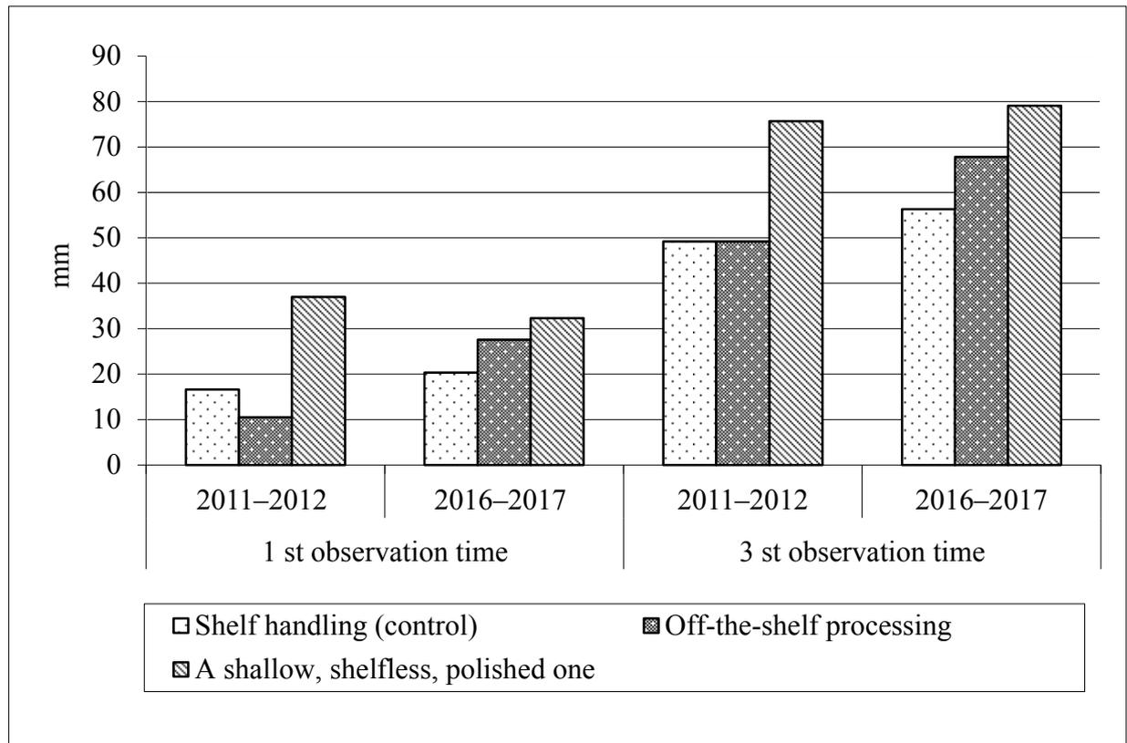
**Fig. 1. Water permeability of black soil typical for different soil tillage systems, mm**
